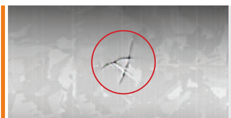
Crack inspection (solar wafer)
